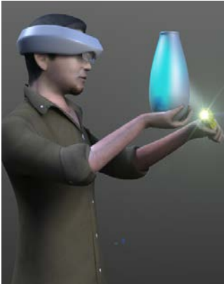
Figure 4: Effect drawing of TranslucentAR. The man wearing HMD is observing an imitation of vase. In his visual field, he can see the translucent relic and extra text information about the history of this relic. Now he is using a torch to appreciate the translucent vase. With high brightness and penetrability of the torch light, the internal structure can be observed carefully to check cracks and flaws of the jade. The torch light is captured by the cameras in the imitation of vase.
