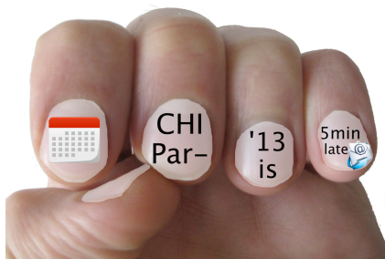
Figure 2: Aligning multiple fingers and selecting a nail with the thumb expands the item, here a calendar event, to all fingers to reveal more information and controls.
